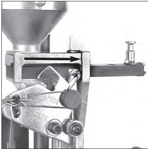
Fig. 52 - This photo shows the powder bar at the end of its travel.
