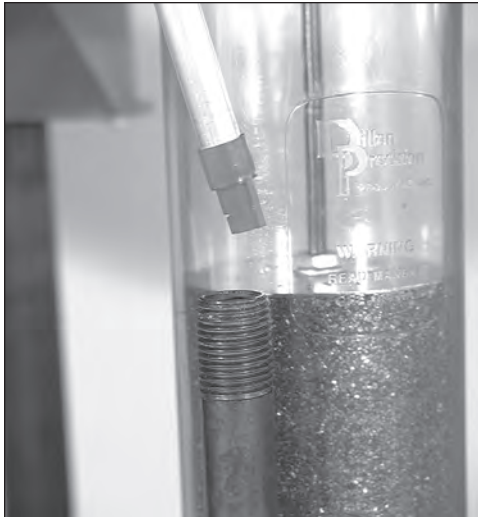
Fig. 32 - Note the shape of the key at the base of the primer magazine tip.
