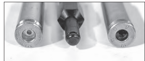
Fig. 59 - Note the difference between the swaged primer pocket (left) and the unswaged primer pocket (right).
