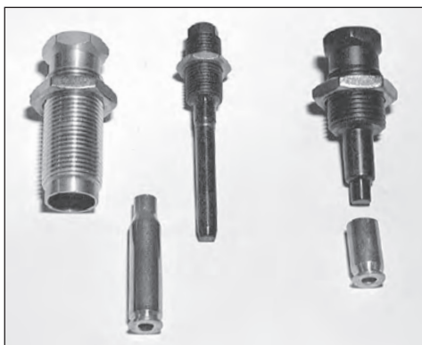
Fig. 15 - Note the difference between the rifle expander (center) and the pistol expander (right).
