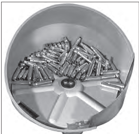
Fig. 24 - The casefeed bowl will hold approximately 500 pistol cases or 350 rifle cases. Do not overload the casefeed bowl.
