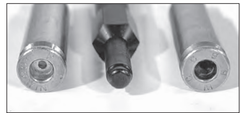
Fig. 31 - Note the difference between the swaged primer pocket (left) and the unswaged primer pocket (right).
