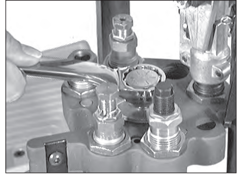
Fig. 36 - To remove the toolhead unscrew the toolhead bolt and remove.
