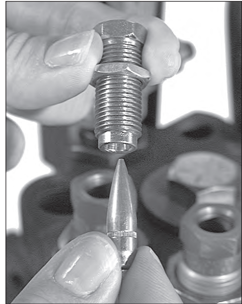
Please note that every die set includes seating stems to fit most common bullet types. Select the appropriate seating stem for the bullet type you are loading.
