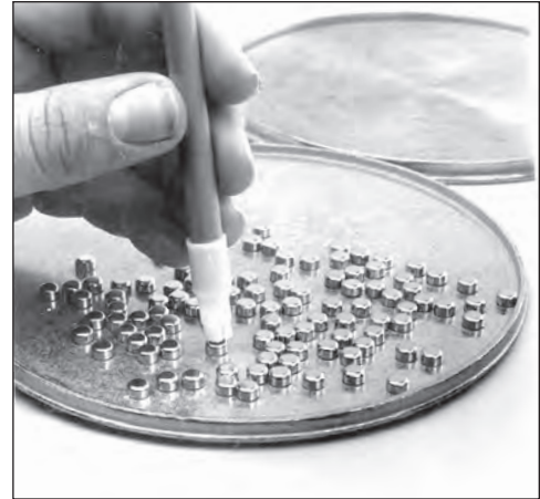
Fig. 21 - All of the primers must be shiny side up.
